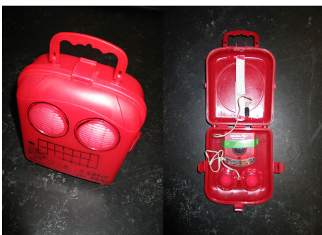
Figure 2 Dream Trunk: an early stage model of the Dream Trunk that reveals a simple technological solution based on a digital sound recorder and player
